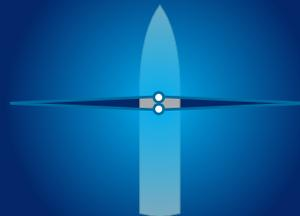
Two 180° systems mounted forward and aft, providing 360° coverage when a single 360° unobstructed view is not possible.
