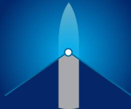
Single 225° system when the top position on the mast is unavailable and the area of interest is only forward.
